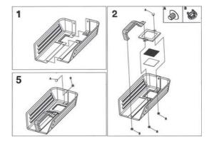
5. Finally use the last plastic screw and clip as shown to fix the two halves of the shield together.
