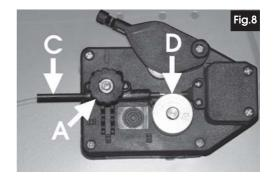
Reposition the pressure roller bracket and securing knob (A) and tighten slightly.
